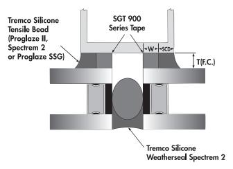
T = Sealant/Tape Thickness 1/4" min. (6.35mm) SCD= Surface Contact Depth 1/4" min. (6.35mm) W = Width of Tape (Adhesive side)
