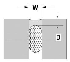
Expansion Joints- The minimum width and depth of any sealant application should be 1/4" x 1/4" (6 mm x 6 mm). The depth (D) of sealant may be equal to width (W) of joints that are less than 1/2" wide.
